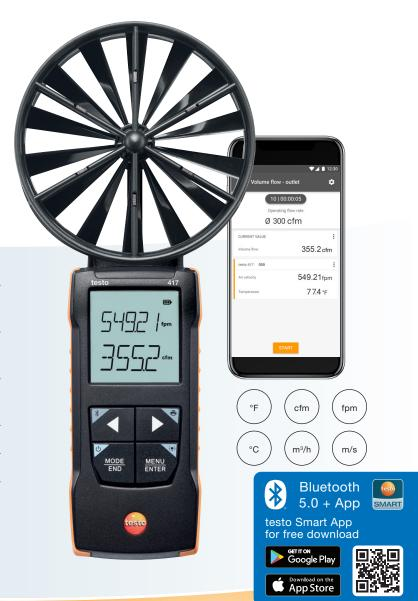
The compact testo 417 4 inch vane anemometer was developed to ensure precise results when measuring air inlets and outlets of **air conditioning and ventilation systems**. Time and point average values as well as the volume flow are automatically calculated in the instrument and shown on the display.
