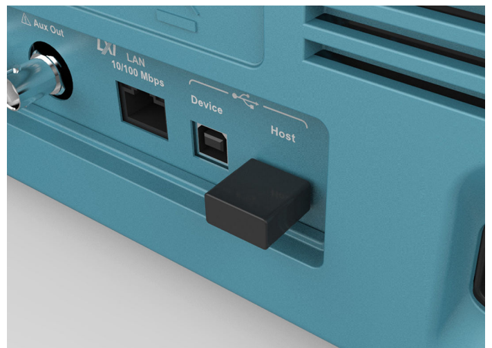
Figure 10: Wi-Fi adapters are configured through integrated setup menus and support seamless wireless communications
