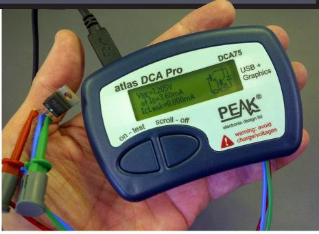
Detailed component information on your PC, complete with curve tracing functions.
