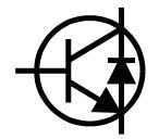
For NPN transistors, the anode of the diode is connected to the emitter of the transistor. For PNP transistors, the anode of the diode is connected to the collector of the transistor.
