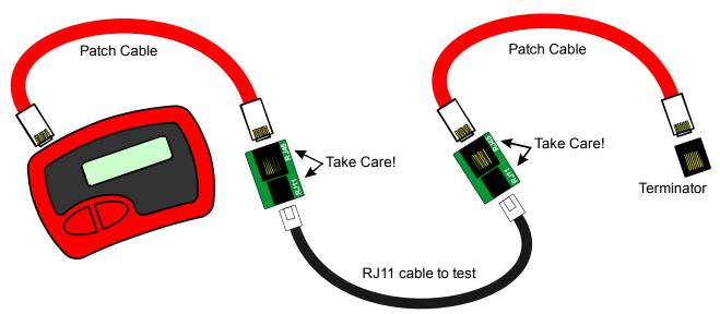
It is common for RJ11 terminated cables to be wired in a mirrored format although straightthrough connections are also in use.
