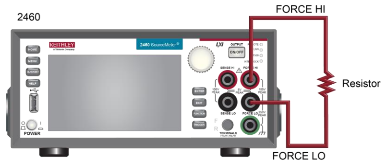
Figure 19: 2460 2-wire front-panel connections
