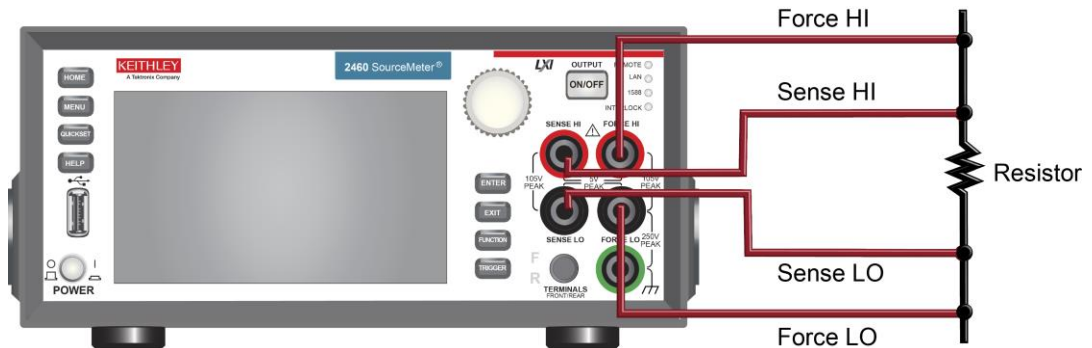
Figure 51: 2460 4-wire connections to the front panel
