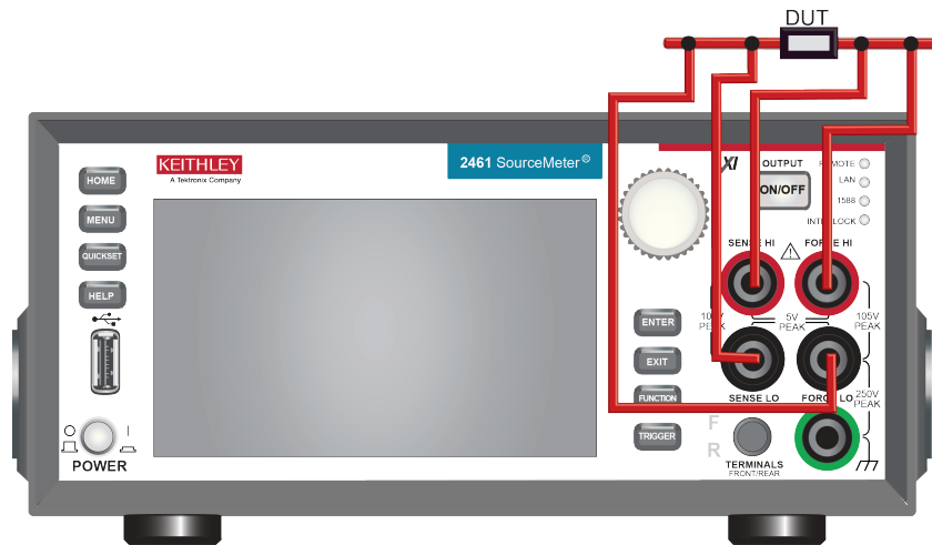
Figure 61: 2461 4-wire sense front-panel connection
