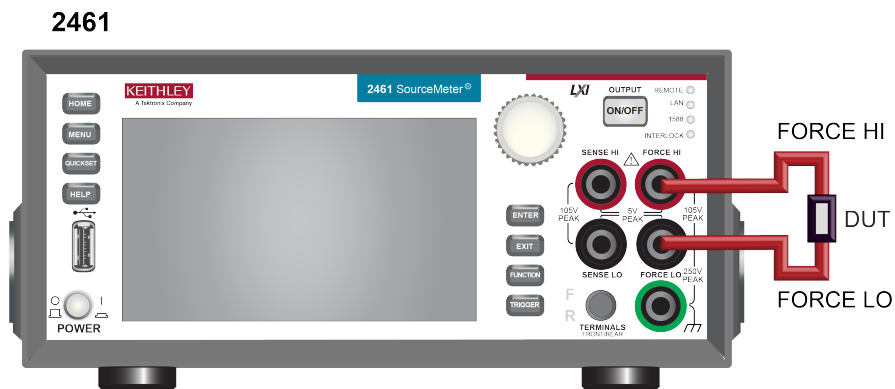
Figure 59: 2461 2-wire rear-panel connections
