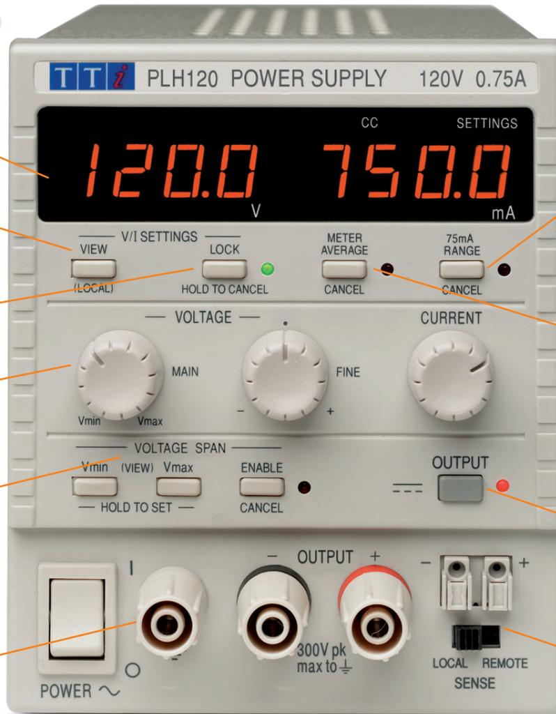
Low current range gives 0.01mA meter resolution and finer low current setting.
