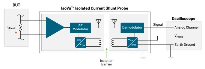
Complete galvanic isolation between the probe tip and the oscilloscope eliminates ground loops and delivers extraordinary common mode rejection.
