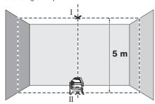
Rotate the measuring tool 180°. Position it so that the centre of the lower laser point is on the point II which has already been marked. Allow the measuring tool to level. Mark the centre of the upper laser point (point III).
