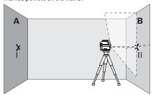
Without changing the height, turn around the measuring tool by 180°. Direct it against the wall A in such a manner that the vertical laser line runs through the already marked point I. Allow the measuring tool to level in and mark the cross point of the laser lines on the wall A (point III).
