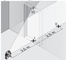
Position the measuring tool on the other side of the door opening directly behind point II. Allow the measuring tool to level in and align the vertical laser line in such a manner that its centre runs exactly through points I and II.
