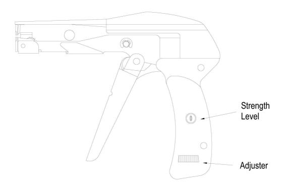
Install Cable Tie From 2.2 To 4.8mm Width, And Up To 1.6mm Thickness
