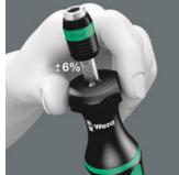
Simple setting of the required torque by hand. Easy-to-read scale value. Measurement accuracy is ± 6 % in accordance with the standard EN ISO 6789. Distinctly audible and noticeable excess-load signal when the pre-set torque is reached.
