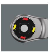
The dual-ratchet-teeth design means that a 76 fine-toothing division can be achieved from the 38 robust teeth with a return angle of only 4.7°.
