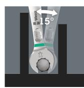
The Joker 6003 ring spanner with its special mouth geometry - a mouth side pivoted by 7.5° and the double hexagon geometry doubles the placement possibilities when repeatedly turning the wrench 180° around the longitudinal axis. Bolts and screw heads can be "taken" every 15°. The Joker 6003 will automatically find the respective placement point after every turn.
