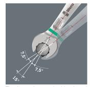
Thanks to the mouth side pivoted by 7.5°, double hexagon geometry and an adjusted application method (placement – screwdriving turning - replacement screwdriving - turning, etc), even screwdriving challenges allowing a pivoting angle of less than 30° can be solved.
