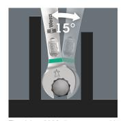
The Joker 6003 ring spanner with its special mouth geometry - a mouth side pivoted by 7.5° and the double hexagon geometry doubles the placement possibilities when repeatedly turning the wrench 180° around the longitudinal axis. Bolts and screw heads can be "taken" every 15°. The Joker 6003 will automatically find the respective placement point after every turn.
