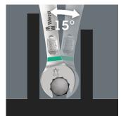
The Joker 6003 ring spanner with its special mouth geometry - a mouth side pivoted by 7.5° and the double hexagon geometry - doubles the placement possibilities when repeatedly turning the wrench 180° around the longitudinal axis. Bolts and screw heads can be "taken" every 15°. The Joker 6003 will automatically find the respective placement point after every turn.
