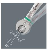
Thanks to the mouth side pivoted by 7.5°, double hexagon geometry and an adjusted application method (placement – screwdriving – turning – replacement – screwdriving – turning, etc), even screwdriving challenges allowing a pivoting angle of less than 30° can be solved.
