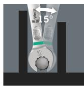
The Joker 6003 ring spanner with its special mouth geometry - a mouth side pivoted by 7.5° and the double hexagon geometry doubles the placement possibilities when repeatedly turning the wrench 180° around the longitudinal axis. Bolts and screw heads can be "taken" every 15°. The Joker 6003 will automatically find the respective placement point after every turn. For pivoting angles under 30°
