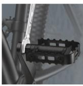
The extra thin pedal wrench (6003 Joker 15 Pedal) is ideal for narrow installation spaces
