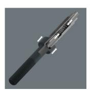
Four screw sizes can be operated with the 4-in-1 bits 9506 and 9507. The 4-in-1 bit 9506 for four sizes of hexagonal socket screws (3.0; 4.0; 5.0; 6.0), the 4-in-1 bit 9507 for three sizes of hexagonal socket screws (2.5; 5.0; 6.0) and one size of TORX® screws (TX 25). In order to use the larger profile, continuously press against the spring tension screwdriving so that the smaller profile is countersunk and the larger profile can be used.
