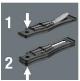
The 4-in-1 bit is clipped into the 9504 tyre lever. The 9505 tyre lever can be attached so that the lever and bit form a compact package.
