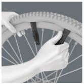
With the glass fibre reinforced plastic tyre levers, the tyres can be safely levered off the rim without damaging the rim. Lift off of the rim with one tyre lever, hook into a spoke and pull off the tyre with the second tyre lever. The two tyre levers can be clicked together and are therefore not lost individually.
