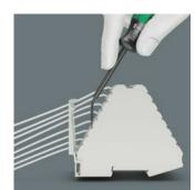
Terminal blocks hold the wire ends mechanically. The force required for this is applied by a spring in the case of tension spring terminals. The spring must be opened by a tool in order to be able to insert the wire ends. The special actuation tools from Wera allow operating the tension spring terminals - even in tight spaces such as switch cabinets. The curved blade also allows spring terminals to be reached where straight-blade tools cannot be used.
