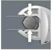
The parallel, smooth jaws of the Joker 6004 VDE offer a seating stress and can thus prevent the nut or screw head from rounding, which can occur when power is transmitted over corners.
