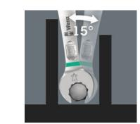
The Joker 6003 ring spanner with its special mouth geometry mouth side pivoted by 7.5° and the double hexagon profile doubles the placement possibilities when repeatedly turning the 180° wrench around the longitudinal axis. Bolts and screw heads can be "accessed" every 15°. The Joker 6003 will automatically find the respective placement point after every turn.
