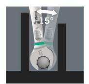
The Joker 6005 double openended wrench with its special mouth design - a 7.5° pivoted mouth and double hexagon geometry - doubles the placement points at a repeated 180° rotation of the wrench around the longitudinal axis. Bolts and screw heads can be engaged every 15°. The Joker 6005 will automatically find the respective placement point after every turn.
