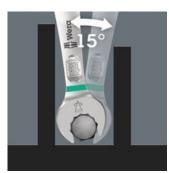
The Joker 6005 double openended wrench with its special mouth design - a 7.5° pivoted mouth and double hexagon geometry - doubles the placement points at a repeated 180° rotation of the wrench around the longitudinal axis. Bolts and screw heads can be engaged every 15°. The Joker 6005 will automatically find the respective placement point after every turn. **Double-hex geometry**
