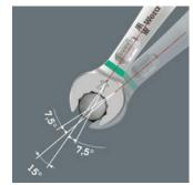
the Thanks to 7.5° pivoted mouths, the double hexagon geometry and an improved application method (placement screwdriving - rotation - replacement - screwdriving - rotation etc), even screwdriving situations that have a pivoting angle of less than 30° can be solved.
