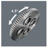
The integrated ratchet with fine toothing (80 teeth) and a return angle of 4.5° eases and accelerates screwdriving without having to reposition the tool.
