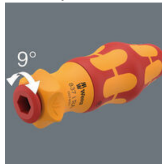
The integrated ratchet with fine toothing (40 teeth and a return angle of 9°) eases and accelerates screwdriving without having to reposition the tool.
