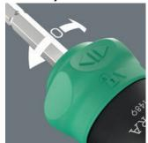
Intuitive switching of the ratchet mechanism. Turn the switch clockwise clockwise for screwdriving; turn it counterclockwise for counterclockwise screwdriving. Use position 0 to deactivate the ratchet mechanism for precise working.
