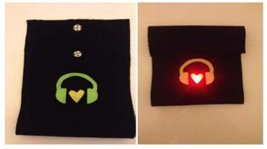
Finish off by sewing up the sides with conventional thread using either a sewing machine or hand sew.
