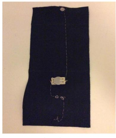
4. Sew from the positive side of the Battery holder to the male part of the press stud above, secure tightly and cut thread.
