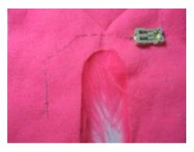
last few stitches need a **large** stitch for the soft switch to lie across. Before making your large stitch, knot the thread for stability, stitch a large stitch and then knot again. This just secures your large stitch firmly in place for the switch to sit on. Make a couple more small running stitches and then fasten off. Your thread may now be cut off.
