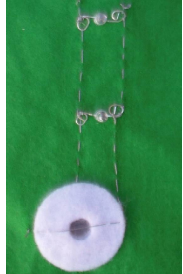
Completed Soft Switch
