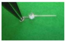
4. Loop the thread through the material and light legs and back through the material. This produces a loop of a smart thread, the needle can then be placed through the loop and pulled tight to produce a knot. Attach two knots, making sure knots are pulled very tight.
