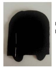
Make sure the positive leg (longest) is pointing up and negative leg is pointing down.
