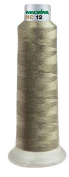
The conductive thread used by Light Stitches is a medium weight and comes on a bobbin of approximately 6M or 150M reel. The thread is much stronger than domestic poly/cotton thread, and somewhat thicker. If using on a machine you may wish to try a larger needle to help with threading up and less chance of fraying by being caught on the point of the needle.
