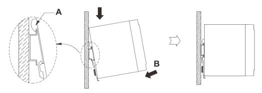
Firstly hang A part on the top of Rail as shown in below, then push the power supply into B direction to fix it.
