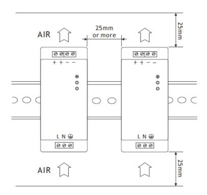
Mounting method should be considered with airflow. Leave enough space between the units
