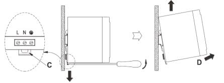
Remove the power supply to D direction, pulling C part by using tools, such as a screwdriver, to downward direction.
