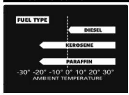
Although this heater operates with diesel fuel, when the temperatures are below 0°C, diesel additives are required to maintain the diesel's viscosity. Typically diesel can cloud in freezing conditions and will start to gel. You will need additives for your fuel in these conditions. Kerosene/Paraffin does not start to gel until the ambient temperature is around -40°C.
