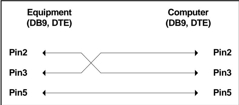
Figure 4: DB25 to DB9 / DB9 to DB9 Wiring Configuration
