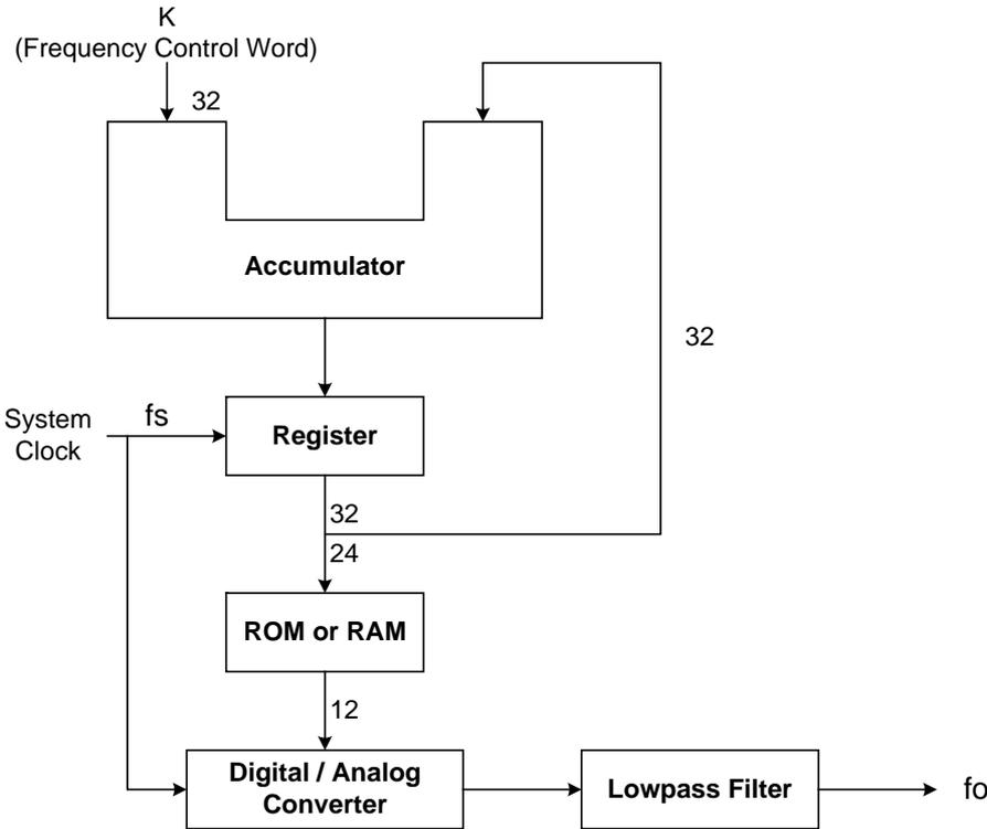
A DDS frequency synthesizer consists of a phase accumulator, a lookup table (ROM or RAM), a Digital-to-Analog Converter (DAC), and a Lowpass Filter (LPF). The amount in a phase accumulator is controlled by the frequency control word (K), which will be added by 1 after each system clock cycle(=1/fs). The output of the accumulator is used to position the data in the Table ROM (or RAM). The digital data will then be converted into a smooth analog waveform after passing through the DAC and LPF.
