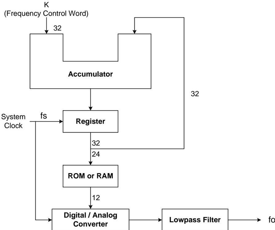
A DDS frequency synthesizer consists of a phase accumulator, a lookup table (ROM or RAM), a Digital-to-Analog Converter (DAC), and a Lowpass Filter (LPF). The amount in a phase accumulator is controlled by the frequency control word (K), which will be added by 1 after each system clock cycle(=1/fs). The output of the accumulator is used to position the data in the Table ROM (or RAM). The digital data will then be converted into a smooth analog waveform after passing through the DAC and LPF.
