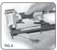
Close the magazine and ensure the latch correctly engages and is fully secure.
