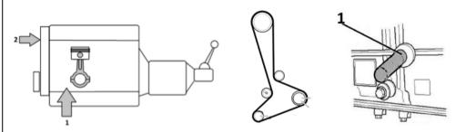
Note: Remove Exhaust Camshaft Oil seal.
