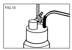
If pumping water from a sandy or muddy floor bed, the pump can be suspended using a rope or chain (not supplied) fixed to the handle. DO NOT use any of the electrical cables for this purpose.
