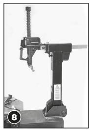
Tilt pneumatic column backwards and hold in place while you insert head and then secure the compression spring with cap and hex. head screw.
