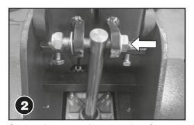
Connect the pneumatic ramp to the column with nut and bolt and washer supplied.
