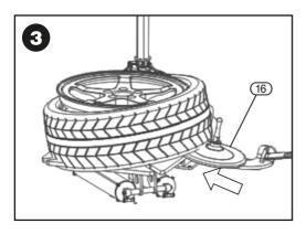
Swing in the lift disc 16 under the tyre, (ensure it does not touch the wheel rim).
