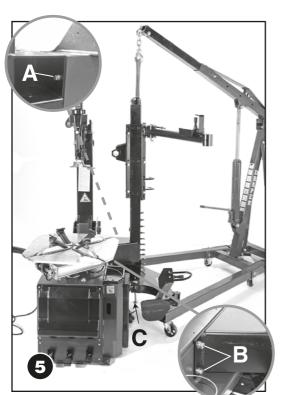
Using an engine crane position and bolt the assist arm column to the main body with 3 bolts supplied (2 at side, 1 from the back) and adjust the support leg C to meet the floor.
