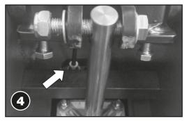
Connect the pneumatic column air pipe.
