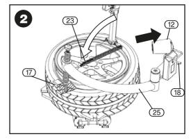
With the tyre lever (23) still under the bead remove roller (12).
