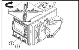
Press pedal ② 3 to 5 times = 1 drop of oil into pneumatic lubricating cylinder.
