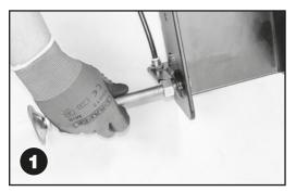
Screw the support leg into the base of the assist arm.
