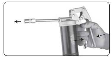
Use above procedure to exchange grease cartridges. If changing grease types, be sure to clean out face of grease cartridge mating face and use new grease to expel old grease before use. After initial assembly, there is no need to remove the nozzle assembly.
