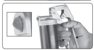
Screw outlet nozzle into main pump head in a clockwise direction until tight. PTFE tape can be used for this joint if required.
