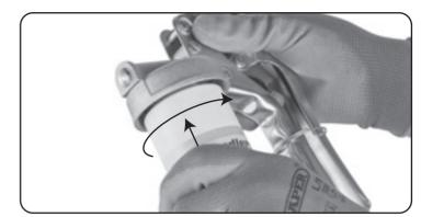
Screw steel barrel over cartridge, into pump head. Be careful not to cross thread it. (Note: steel barrel is not supplied or required for Draper Stock No.16157).
