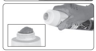
Screw cartridge firmly into pump head in a clockwise rotation until it stops. Do not over tighten.
