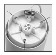
Bring the 2 halves of the base sections together whilst ensuring the power cable passes though the hole created when assembled. Secure the assembled base to the fan body using the three screws provided.
