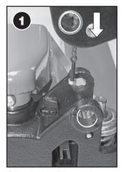
Offer the handle up to the piston's pre-drilled holes.
