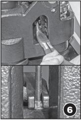
Adjust the control lever to the 'Lift' position. This will extend the length of the chain and adjusting bolt/nut. Lift the lever plate and slide the adjusting bolt through the slot.
