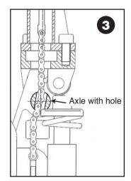
Adjust the control lever to the lower position. Then feed the chain and adjusting bolt/nut through the axle pin.
