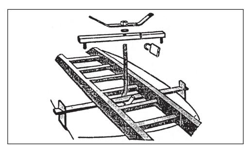
Assemble components as shown above to make two rack clamps (padlock not included).
