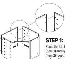
Place the left back panel (item 1) and right back panel (item 2) together on a level surface. Attach right back panel to left back panel by engaging the holes on the left back panels with the corresponding hooks on right back panel.
