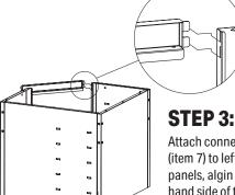
Attach connecting beam (item 7) to left and right side panels, algin the tabs on right hand side of the connecting beam with the holes on right side panel, slide the connecting beam together with tabs and holes fully engaged. Repeat the step above to complete another side assembly.
