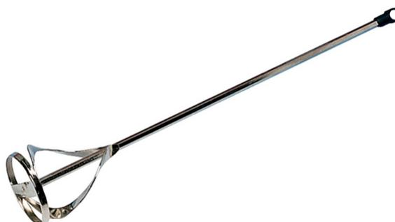
**Features & Benefits** ~ Nickel plated steel construction for strength & easy cleaning ~ Suitable for use with electric drills at speeds between 200 ~ 700 rpm ~ Length: 620 mm ~ Mixer diameter: 100 mm ~ Drive: 10 mm ~ Flow direction: depending on right or left use ~ Capacity: 5 ~ 10 kg, depending on material
